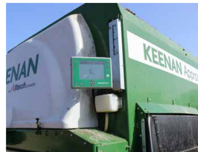
The diet feeder is equipped with the latest KEENAN Controller, which wirelessly sends all mixing and feed-out data back to the InTouch nutrition centre for analysis.
